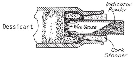
FIG. 2 Longitudinal Section Showing Construction of Desiccator and Shaker
